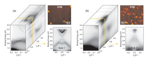
FIG. 3. (Color online) The effect of defect creation on the surface. Differences between (a) a pristine surface and (b) a sputtered surface. Each panel shows a 3D representation of the electronic structure obtained by taking data as a function of photon energy. Images corresponding to the center of the bulk Brillouin zone are shown separately. The STM images of the surface were measured using a voltage and tunneling current of 1.84 V and 0.18 nA in (a) and 1.68 V and 0.45 nA in (b).
