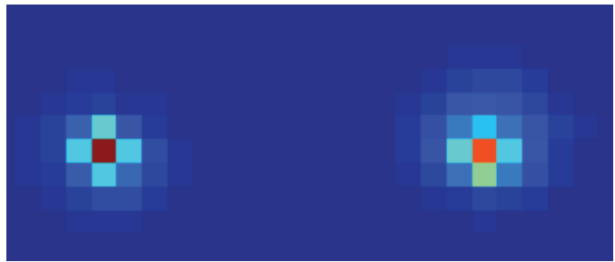
Figure 5 (below). Figure 15 from the Kepler Instrument handbook (KSCI-19033) showing the PSF (or PRF) for a point source in the focal plane (detected by use of Kepler).
